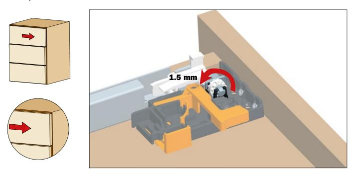
We suggest to make the sideways adjustment on both clips in the same way to keep the runners parallel and sliding.
