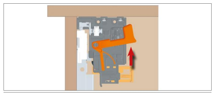
**SIDE REMOVAL:** position the hands under both sides of the drawer and operate on the orange levers, as indicated in the drawing, sliding the drawer forward.
