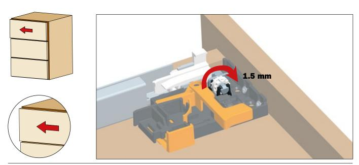
Rotate the white wheels towards the back of the drawer to adjust right.
