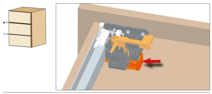
Push the lever **towards the outside of the drawer** to achieve the height adjustment. This operation is tool free.
