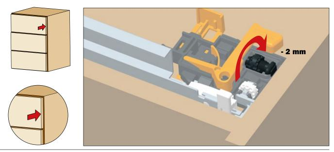
Rotate the **black** wheel **towards the ouside of the drawer** to **increase** the gap between the front and the side.
